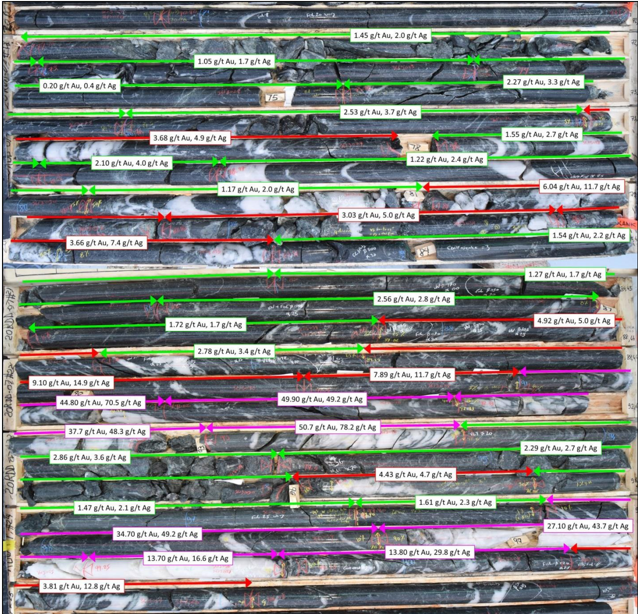
Figure 8: Photographs of core from drill hole 20RDD007 with gold and silver assays.
