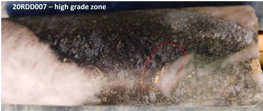
Visible gold associated with quartz-calcite veining hosted within a biotite-calcite +/- silica altered diorite
