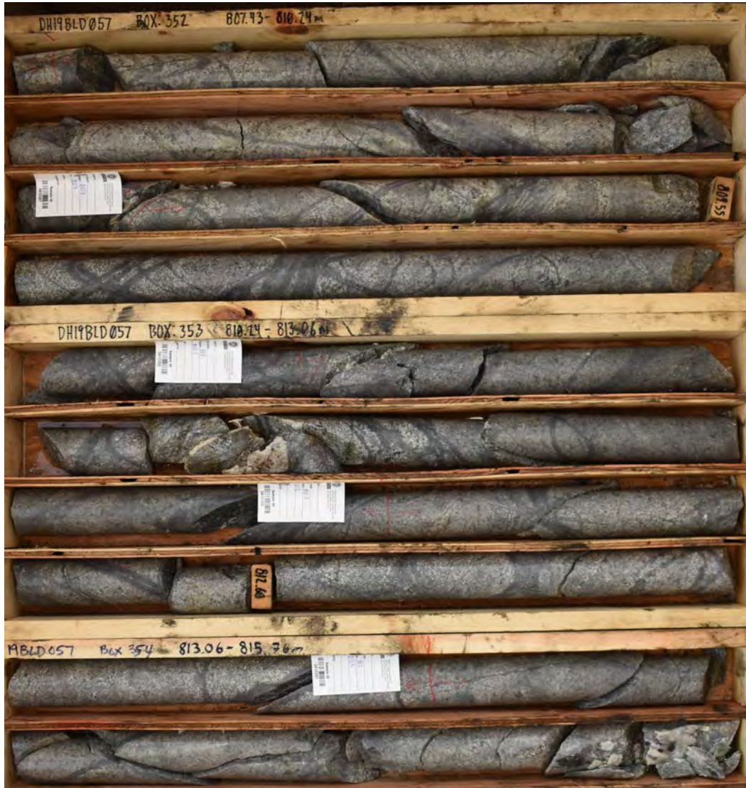
19BLD057 @ 808-816m: felsic intrusive with intense QSP alteration and dark grey qtz-py "D" veining, increasing down hole, no notable assay results
