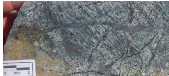
19WTD046 @ 79m: Intrusion breccia, dark grey qtz-mo stockwork veining, chlorite-epidote-K-spar altered
