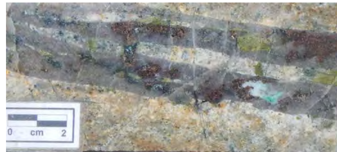
19WTD046 @ 98m: Quartz latite, qtz-gar-ep-mag-mal vein, quartz-sericite-chlorite alteration
