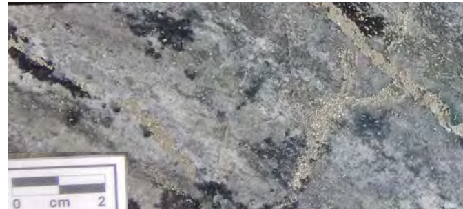
19BLD057 @ 808-816m: felsic intrusive with intense QSP alteration and dark grey qtz-py "D" veining, increasing down hole, no notable assay results
