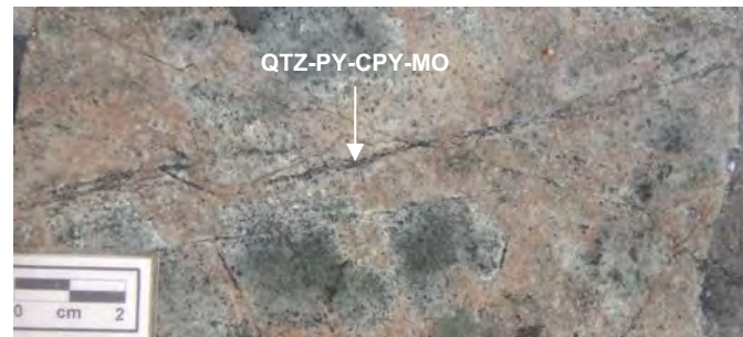
19ETD050 @ 215m: Intrusion breccia, dark grey qtz-py-cpy-mo veinlets, , sericite-chlorite-magnetite altered quartz-latite clasts within strong K-spar altered matrix
