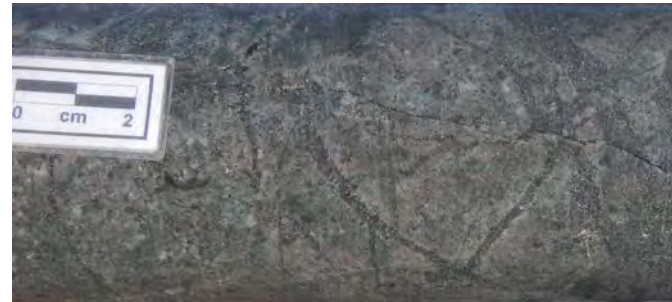
19ETD050 @ 138m: Quartz-monzonite porphyry, dark grey qtz stockwork veining with K-spar alteration selvages, strong py-cpy disseminations
