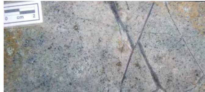
19WTD046 @ 68m: Quartz latite, dark grey qtz stockwork veining, K-spar selvedge grading to chlorite-sericite-pyrite-magnetite alteration
